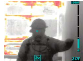
Same picture with 2X Digital Zoom activated showing low-sense imagery on the display of an E5200HD 2 TIC
